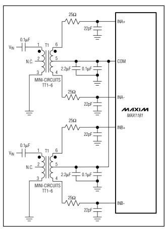
Figure 6. Transformer-Coupled Input Drive
