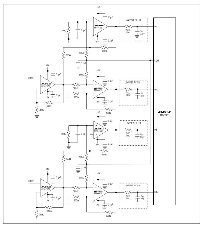
Figure 5. Typical Application for Single-Ended-to-Differential Conversion
