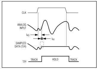
Figure 9. T/H Aperture Timing
