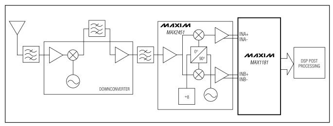
Figure 8. Typical QAM Application, Using the MAX1181
