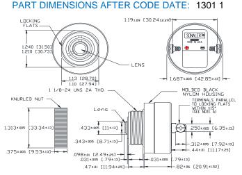
NOTE A: TERMINALS-032 BRASS TIN PLATED, TAPPED FOR #6-32 SCREW. TWO #6-32 NICKEL PLATED BRASS SCREWS INCLUDED. WILL ACCEPT 1/4\* QUICK CONNECT. NOTE B: MOUNTING- REMOVE BLACK PLASTIC NUT
