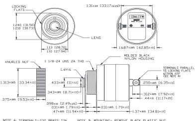
NOTE A: TERMINALS-0.32 BRASS TIN PLATED, TAPPED FOR #6-32 SCREW. TWO #6-32 NICKEL PLATED BRASS SCREWS INCLUDED. WILL ACCEPT 1/4\* OUICK CONNECT. NOTE B MOUNTING- REMOVE BLACK PLASTIC NUT AND INSERT THREADED FRONT THROUGH 1.25\* HOLE PUNCHED IN PANEL, IF DRIENTATION IS NEEDED, NOTE LOCKING FLATS ON DRAWING, SCREW NUT BACK ON. DO NOT OVERTIGHTEN.
