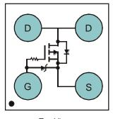
Top View Equivalent Circuit
