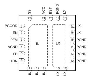
22-Pin 4mm x 4mm QFN (Top View)
