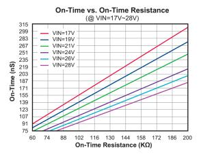
Figure 3. Ton vs R<sub>TON</sub> Curves for AOZ2261QI-11
