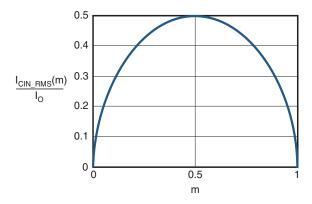
Figure 4. I<sub>CIN</sub> vs. Voltage Conversion Ratio
