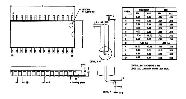
Figure 52. 28-Pin SOIC Package Diagram
