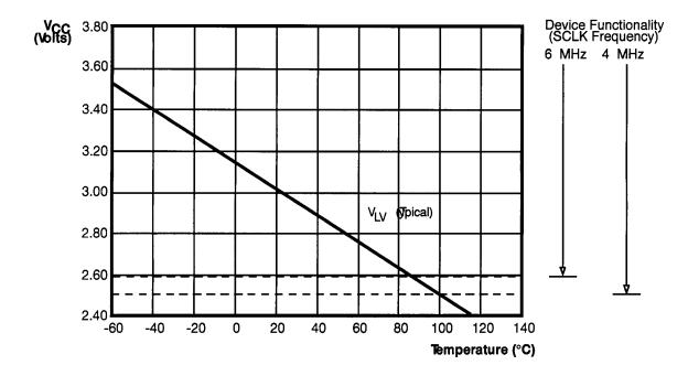
Figure 31. Typical Z86C33/43 Low Voltage Protection vs Temperature
