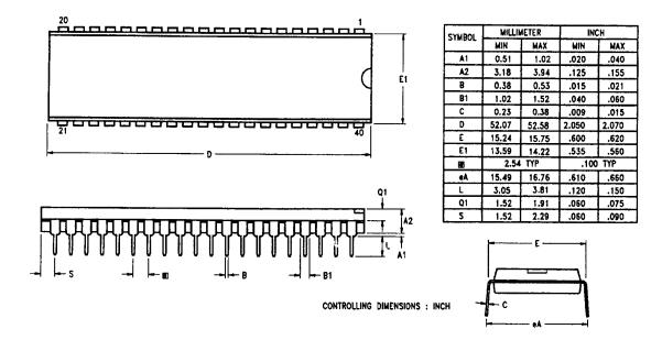
Figure 53. 40-Pin DIP Package Diagram
