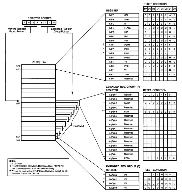
Figure 19. Expanded Register File Architecture
