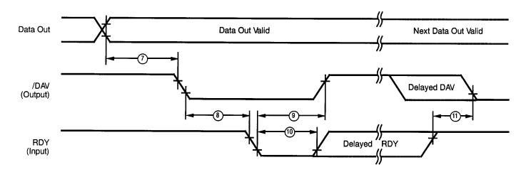
Figure 11. Output Handshake Timing
