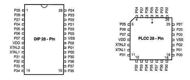
Figure 2. 28-Pin DIP/SOIC Pin Configuration
