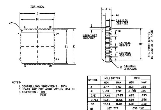
Figure 54. 44-Pin PLCC Package Diagram
