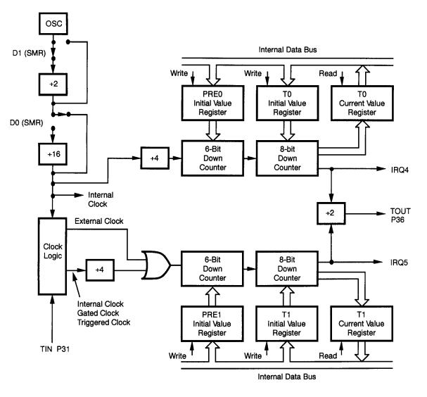
Figure 22. Counter/Timer Block Diagram
