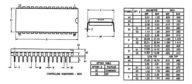
Figure 51. 28-Pin DIP Package Diagram
