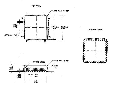
Figure 55. 44-Pin LQFP Package Diagram
