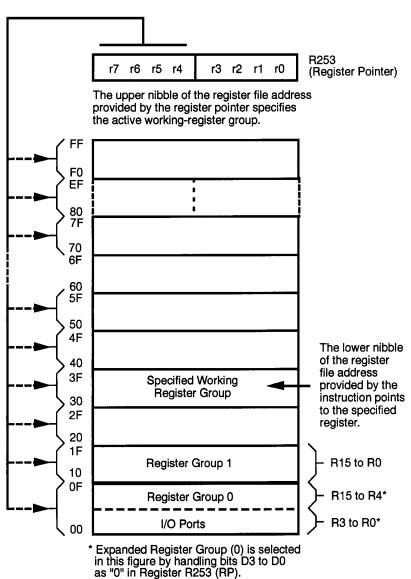
Figure 21. Register Pointer
