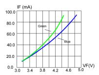
FIG.1 FORWARD CURRENT VS. FORWARD VOLTAGE.
