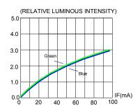
FIG.2 RELATIVE LUMINOUS INTENSITY VS. FORWARD CURRENT
