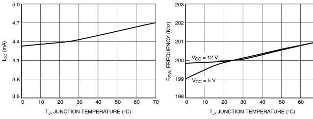
Figure 3. I<sub>CC</sub> vs. Temperature
