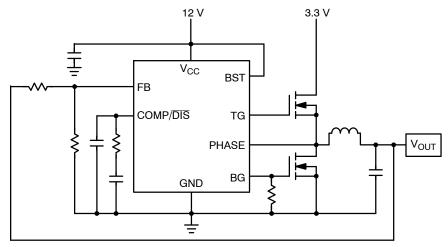
Figure 1. Typical Application Diagram
