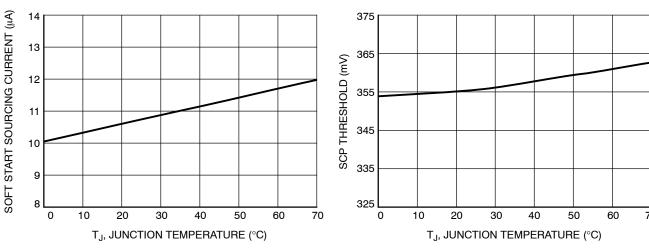
Figure 5. Soft Start Sourcing Current vs. Temperature
