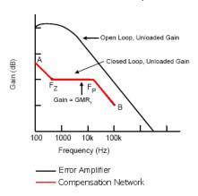
Figure 11. Gain Plot of the Error Amplifier
