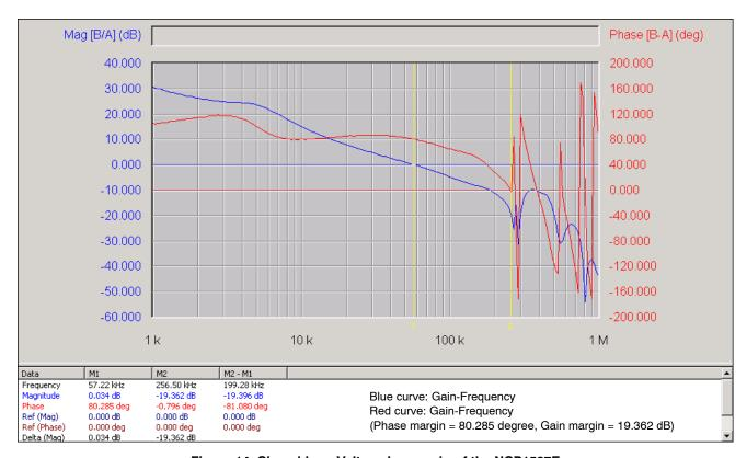
Figure 14. Closed-loop Voltage Loop-gain of the NCP1587E
