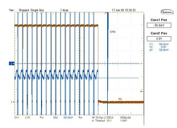
Figure 17. Over Current Protection (12.4 A DC Trip)
