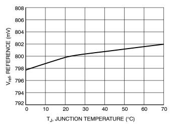
Figure 7. Reference Voltage (V<sub>ref</sub>) vs. Temperature
