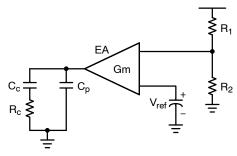
Figure 10. Type II Transconductance Error Amplifier
