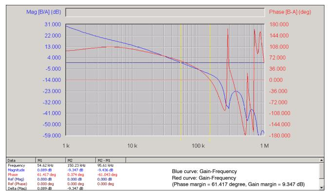
Figure 13. Closed-loop Voltage Loop-gain of the NCP1587E
