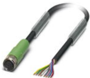
Sensor/actuator cable, 8-position, PUR halogen-free, black-gray RAL 7021, free cable end, on Socket straight M8, cable length: 1.5 m
