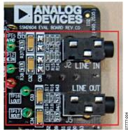
Figure 5. Analog Input/Output Circuitry
