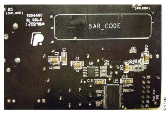
Figure 2. Bottom View of the SSM2604 Evaluation Board
