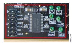
Figure 7. General-Purpose Digital Audio Interface and Buffer
