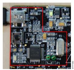
Figure 3. USB Interface Microcontroller
