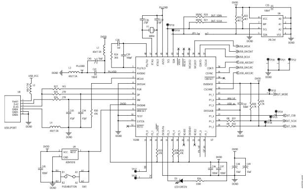
Figure 27. Schematic of SSM2604 Evaluation Board, USB MCU
