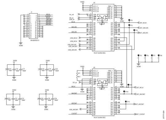
Figure 25. Schematic of SSM2604 Evaluation Board, Digital Buffer
