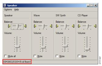
Figure 8. Speaker Control Panel Setting
