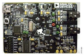
Figure 1. Top View of the SSM2604 Evaluation Board
