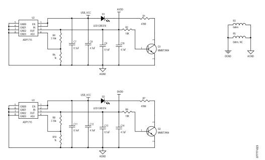
Figure 24. Schematic of SSM2604 Evaluation Board, Power Supply
