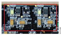
Figure 4. Power Supply Circuitry
