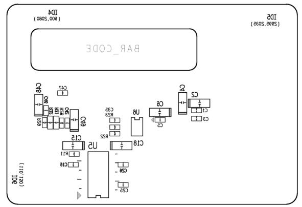
Figure 29. Layout of SSM2604 Evaluation Board, Bottom Layer
