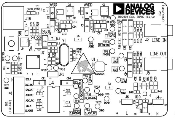
Figure 28. Layout of SSM2604 Evaluation Board, Top Layer
