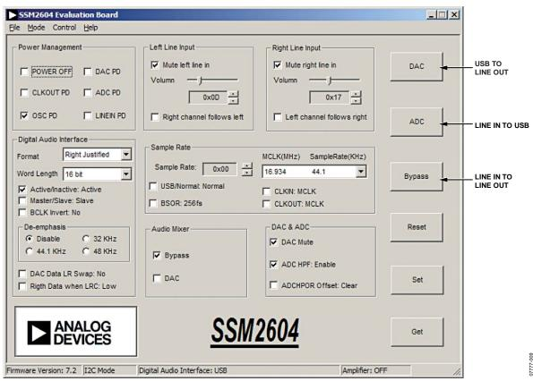
Figure 10. SSM2604 Control Software GUI
