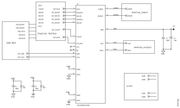
Figure 23. Schematic of SSM2604 Evaluation Board, SSM2604 Chip
