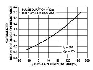
Figure 12. Normalized R<sub>DSON</sub> vs. Junction Temperature
