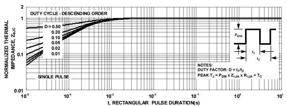
Figure 3. Normalized Maximum Transient Thermal Impedance
