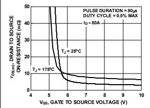
Figure 11. R<sub>DSON</sub> vs. Gate Voltage
