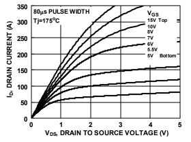
Figure 10. Saturation Characteristics
