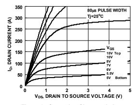
Figure 9. Saturation Characteristics
