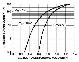
Figure 8. Forward Diode Characteristics
