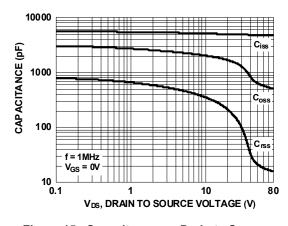
Figure 15. Capacitance vs. Drain to Source Voltage
