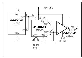
Figure 10. Low-Power, 10-Bit CMOS DAC Connection
