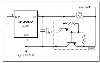
Figure 6. High-Current Precision Supply
