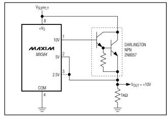
Figure 7. NPN Output Current Booster
