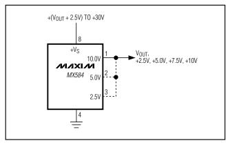
Figure 1. Basic Connection for Positive Outputs
