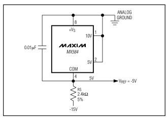
Figure 9. Two-Terminal -5V Reference
