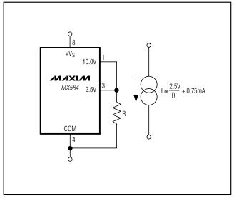
Figure 8. Precision Current Limiter
