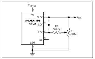
Figure 3. Fine Adjustment of Output Voltage (±200mV)
