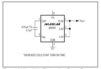
Figure 4. Additional Noise Filtering with an External Capacitor
