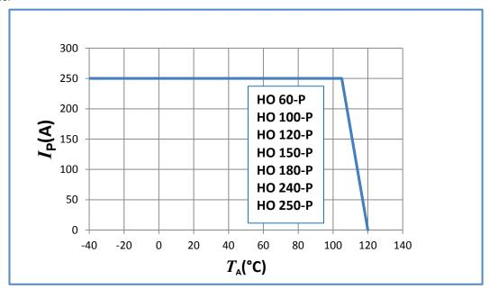
Important notice: whatever the usage and/or application, the transducer primary bar / jumper temperature shall not go above the maximum rating of 120 °C as stated in page 2 of this datasheet.
