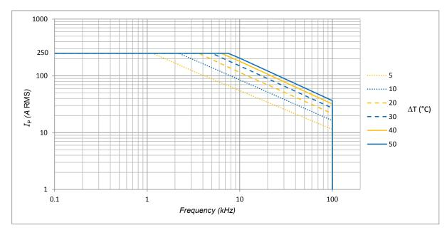
Primary current in A RMS is sine wave.
