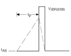
Fig 22b. Unclamped Inductive Waveforms
