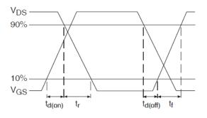
Fig 23b. Switching Time Waveforms
