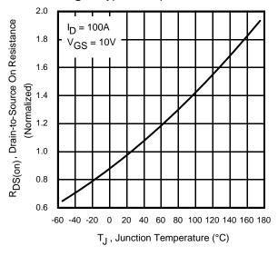
Fig. 4 Normalized On-Resistance vs. Temperature
