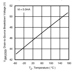
Fig 10. Drain-to-Source Breakdown Voltage
