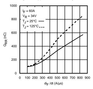
Fig. 21 - Typical Stored Charge vs. dif/dt
