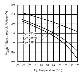
Fig 17. Threshold Voltage vs. Temperature
