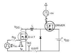
Fig 22a. Unclamped Inductive Test Circuit
