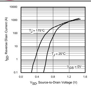
Fig. 7 Typical Source-to-Drain Diode
