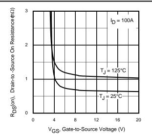
Fig 16. Typical On-Resistance vs. Gate Voltage
