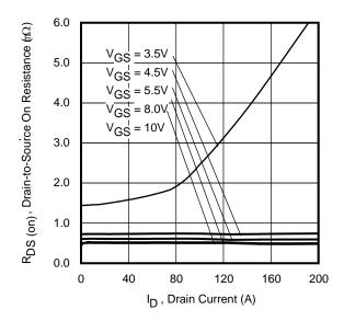
Fig 22. Typical On-Resistance vs. Drain Current
