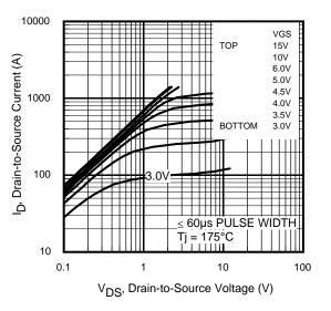
Fig. 2 Typical Output Characteristics
