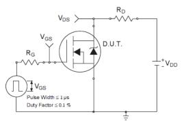
Fig 23a. Switching Time Test Circuit
