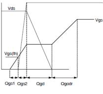
Fig 24b. Gate Charge Waveform
