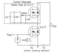
Fig 24a. Gate Charge Test Circuit
